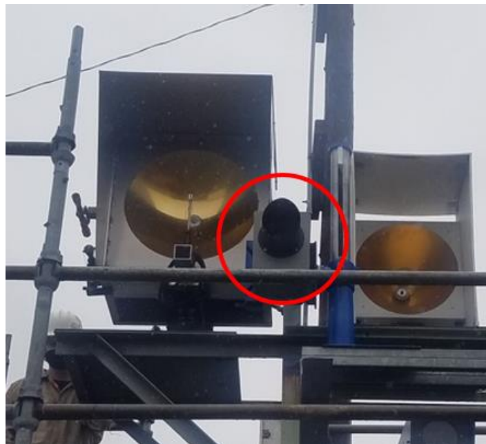
Airoptic Retroreflector Mounted on the Reflector Tower
